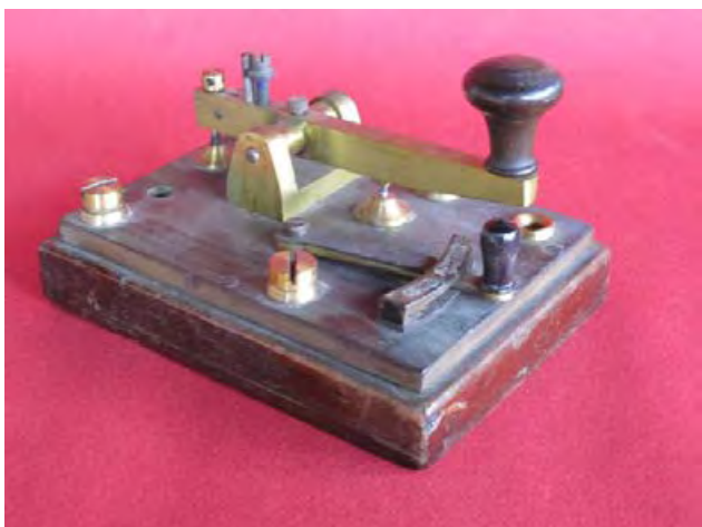
This English key has a changeover switch 'send - receive':
